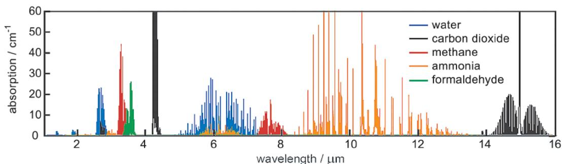
Figure 3. The infrared absorption spectra of several commonly detected gases.
