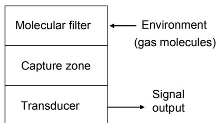
Figure 1. The basic components of a gas sensor.
