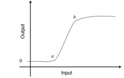
Figure 2. Sketch of a possible input-output relation for a sensor. Point *a* indicates the response threshold and point *b* indicates saturation. The ruling slope of the line connecting *a* and *b* is the responsivity, and the difference in their abscissae is the latitude. This diagram does not show more sophisticated performance criteria such as the detectivity.<sup>5</sup>
