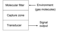
Figure 1. The basic components of a gas sensor.
