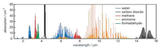
Figure 3. The infrared absorption spectra of several commonly detected gases.
